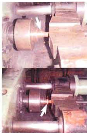
Friction welding process
